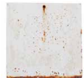
Pinhead dots of rust suggest the aerosol isn't quite as effective as the trigger bottle.
